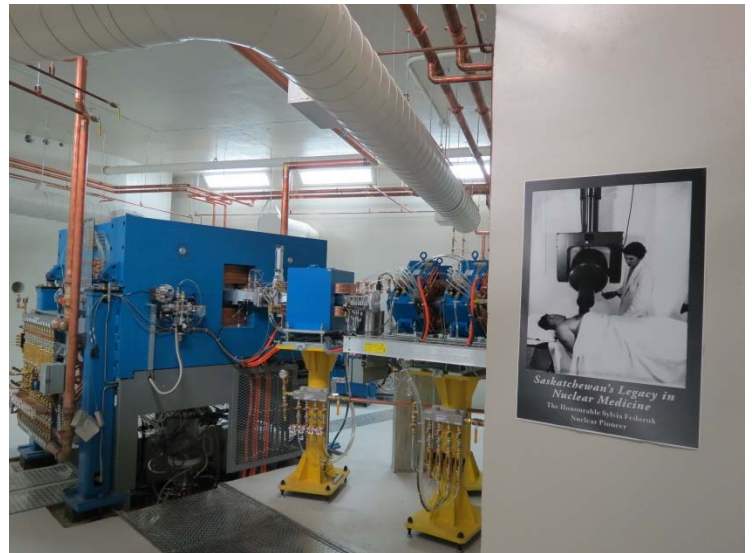
A view of the cyclotron and beamline inside the Saskatchewan Centre for Cyclotron Sciences.
