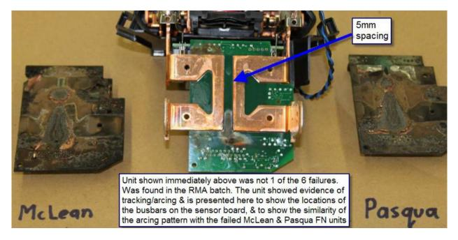
Figure 4: Comparison of burnt boards to RMA board. Source: SaskPower Preliminary Technical Report
