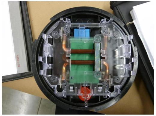
Figure 10: Backplane of Itron internal power board
